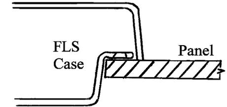
In order to secure the display when flush mounting there is a stainless steel flush mount stirrup provided. This is attached using the plastic m6 studs and nuts provided. Please do not over tighten these mounting nuts as it may distort the case and cause water ingress. It may be easier to thread the power cable through the stirrup and plug it in before mounting the stirrup.
