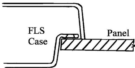
In order to secure the display when flush mounting there is a stainless-steel flush mount stirrup provided. This is attached using the plastic m6 studs and nuts provided. Please do not over tighten these mounting nuts as it may distort the case and cause water ingress. It may be easier to thread the power cable through the stirrup and plug it in before mounting the stirrup.
