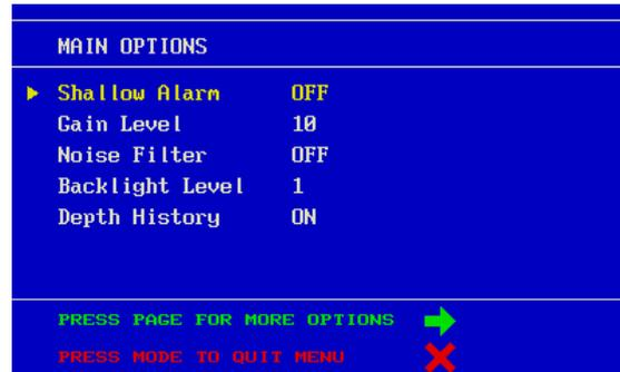
The desired menu option is chosen using the menu key. When the arrow cursor is alongside the appropriate option, pressing the up or down arrow keys changes the setting.
